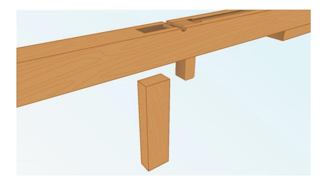
Glue the handle onto the stock behind the trigger. Leave this to dry completely and then strengthen the join with nails.
