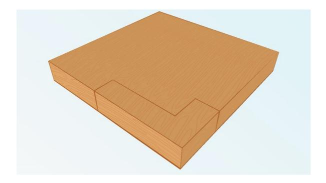
Carve a channel, about  $\frac{1}{8}$  inch long, across the shortest side of your L-shape using a chisel.
